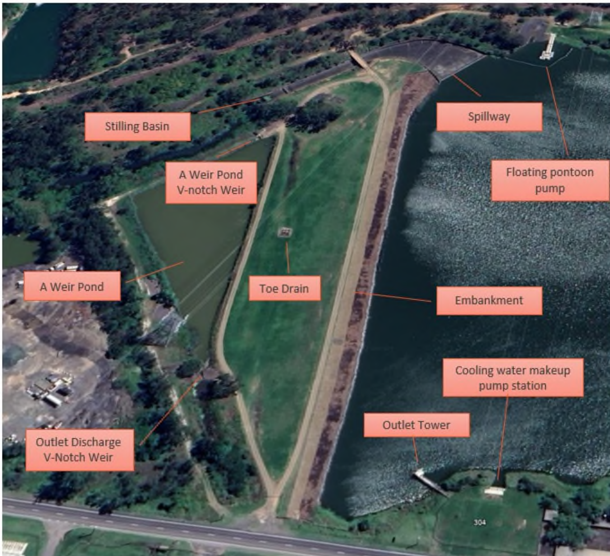
Figure 5: Swanbank Cooling Water Dam - General Arrangement
